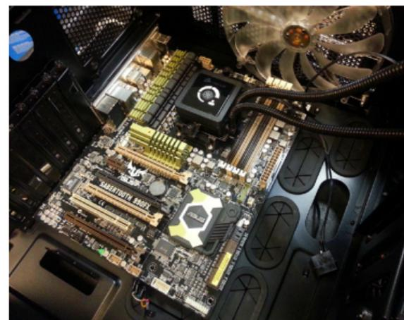
6. Install the graphics card into the x16 PCI Express slot and ensure the appropriate power connectors are used.
